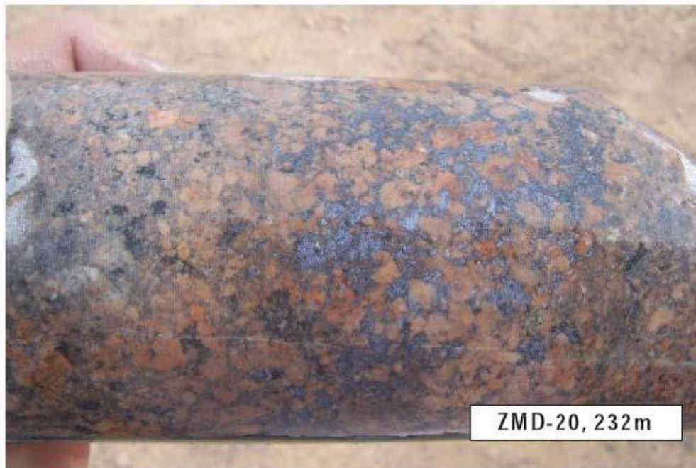
Disseminated molybdenum mineralization (replacing mafic minerals) associated with strong potassic alteration
