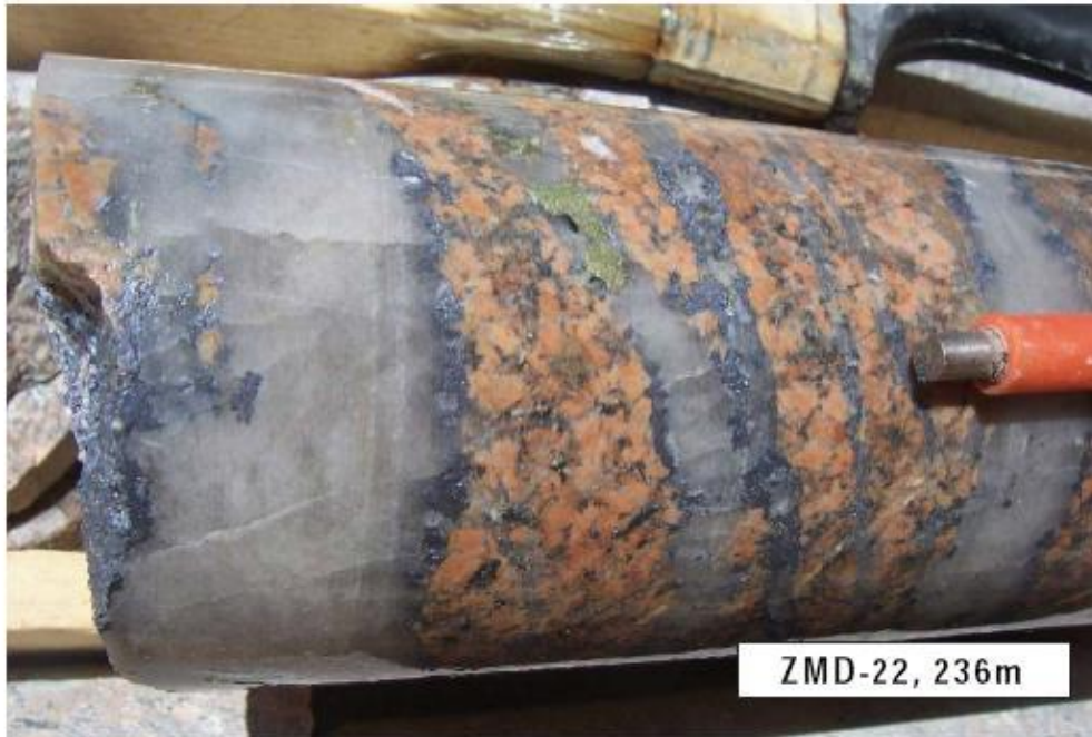
Vein hosted molybdenum mineralization associated with quartz stockwork veins and intense potassic alteration
